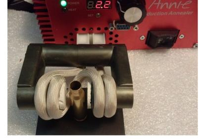
water-cooled and capable of 100% duty-cycle. If you're really into 50BMG or you are cycling thousands of cartridges in an automated setup, this is something you should consider.
